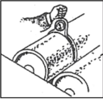
**OPERATION OF THE CALIPER:** The Velocity Steam Caliper is a precision tool which accurately measures roll diameters to within  $1/32''$ . With the ironer operating normally, with or without work being processed, set the Velocity Steam Caliper on the roll and a right angle to the roll shaft, with both sides and top touching the roll. The movable arm automatically adjusts to
